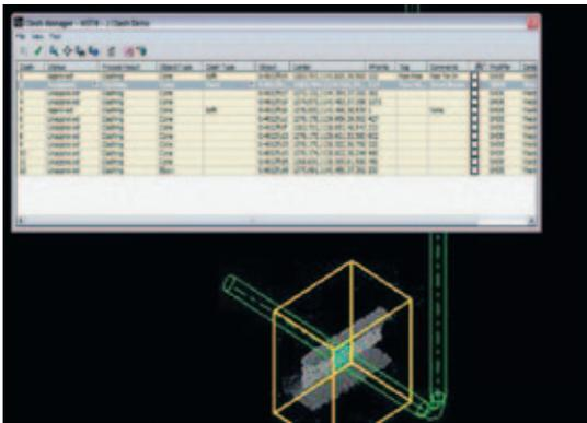
Clash Manager creates a database for managing, tracking, assigning and classifying clashes. A powerful navigation feature lets users easily pull up isolated views of any clash. Here we see a pipe clashing with scanned point cloud data of a beam.
